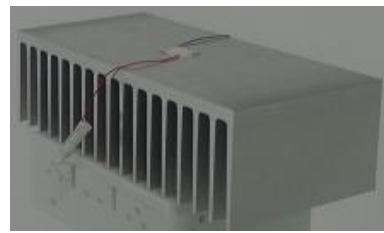
Figure 12. Heat sink with a Thermal Resistance of 0.5^\circ\text{C/W} (150 x 294 x 90 mm)
